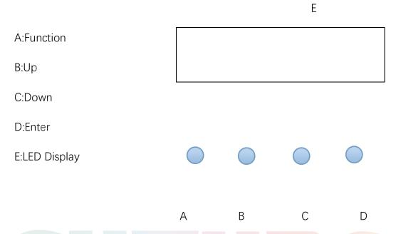
Instructions:Press the function key A cycled out the eight different function effects, digital tube first two digits on behalf of which the current function (see menu). The last two digits represent the functions in which the address code or speed parameters. Press the B or C key to modify the parameter values. Press the D key to confirm.
