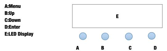
Instructions:Press the function key A cycled out the eight different function effects, digital tube first two digits on behalf of which the current function (see menu). The last two digits represent the functions in which the address code or speed parameters. Press the B or C key to modify the parameter values. Press the D key to confirm.
