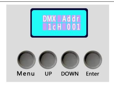
Instructions:Press the function key MENU cycled out the eight different function effects, digital tube first two digits on behalf of which the current function(see menu). The last two digits represent the functions in which the address code or speed parameters. Press the UP or DOWN key to modify the parameter values. Press the ENTER key to confirm.
