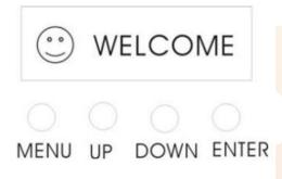
The Control Panel shows the current state of the unit. It is used to select the operating mode, as well as the sub-features. For a detailed layout of the control panel functions, please see the "menu map" section on the following page.
